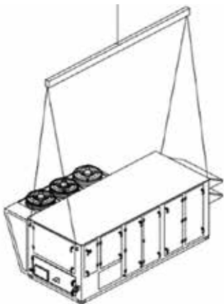
Lifting Details for RV/E 20, 40, 85, and RVC 40, 85. Applies to units with or without side air return Lift from the top of the unit 4 lifting points.
